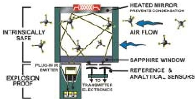
**Figure 3 - Infrared Sensor**
