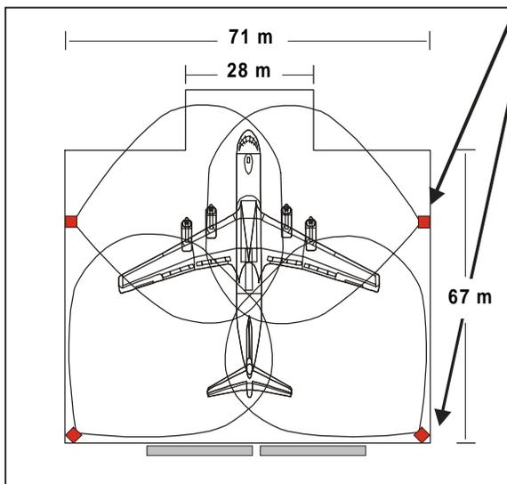
**Underwing Coverage using (4) Model FV-20 UV-IR detectors**
