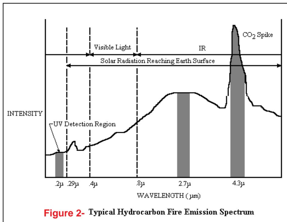
**Figure 2- Typical Hydrocarbon Fire Emission Spectrum**
